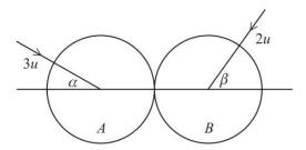
After the collision, the velocity of B is in the direction of the velocity of A before the impact.
