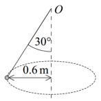
(a) Show that the tension in the string is 22.6 N, correct to three significant figures.
