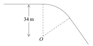
Find the greatest speed at which the van can travel around the bend without causing the parcel to slide.
